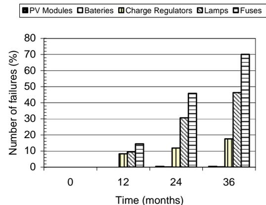
Fig. 4 Number of accumulated failures recorded by the O&M technician during last three years operation.
