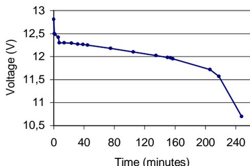
Fig. 5 Discharge curve of one of the local batteries (110 Ah) tested, with a discharge current of 5 A. The real capacity measured was 23 Ah.
