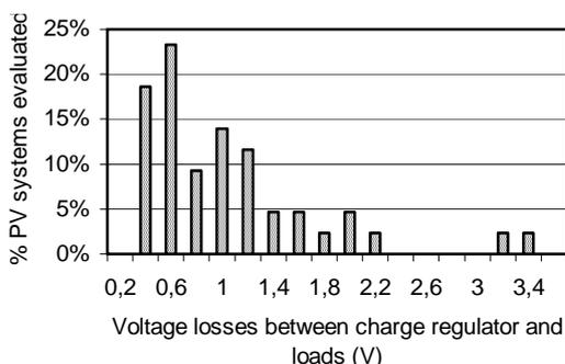
Fig. 6. Frequency of voltage drop between charge regulator and lamps measured.
